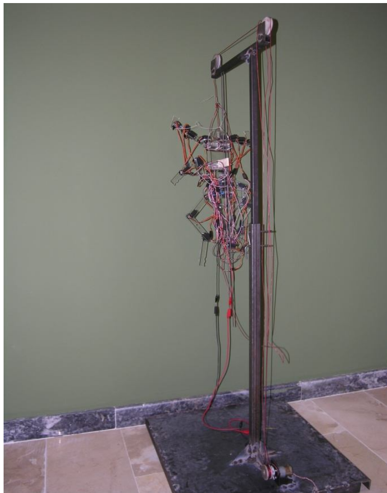
Figure 5.21 A view of the cockroach biorobot with climbing platform
