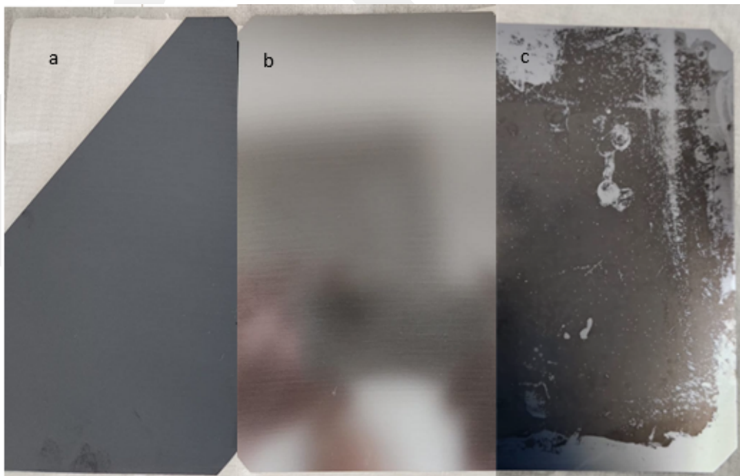
Figure 3.43 Visual comparison of different wafer surfaces: (a) Conventionally textured wafer, (b) SDR wafer, (c) Wafer processed via the SS-INH-PCE method.
