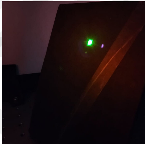
Figure 3.27 Visual observation of residual 1064 nm infrared beam (unfocused) alongside the aligned 532 nm green beam.
