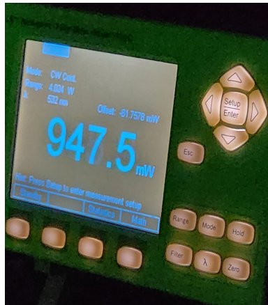
(a) Measured laser power at the source (Newport 1936-C): 947.5 mW.
