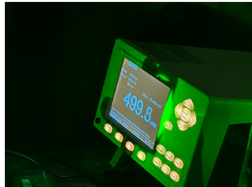
(b) Measured laser power at the wafer surface: approximately 500 mW.
