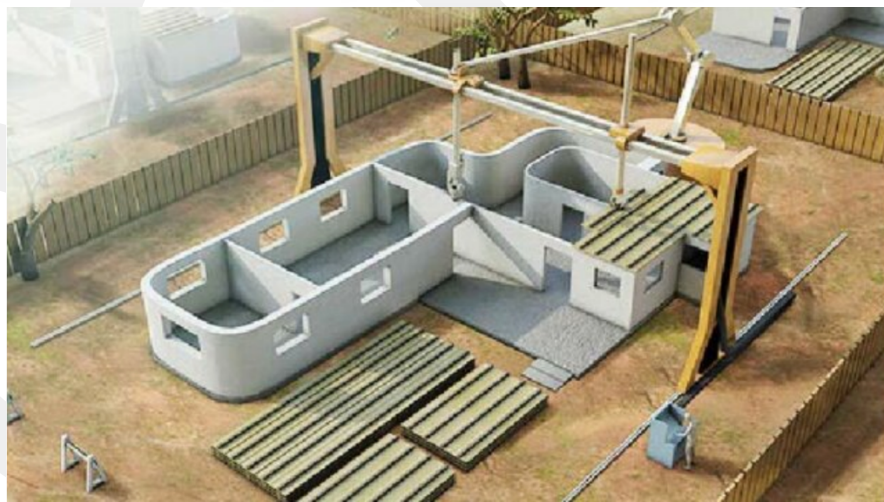
Figure 2.5: Contour crafting Machine (Photo courtesy of Sagheer A. Ranjha).
