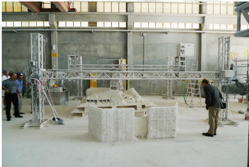
Figure 2.7: D-Shape printing Machine (Photo courtesy of Adlughmin).
