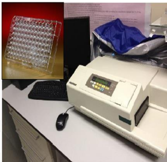
Figure 3. Multi-mode plate reader with 96 well plate (Molecular Devices Spectramax M2)
