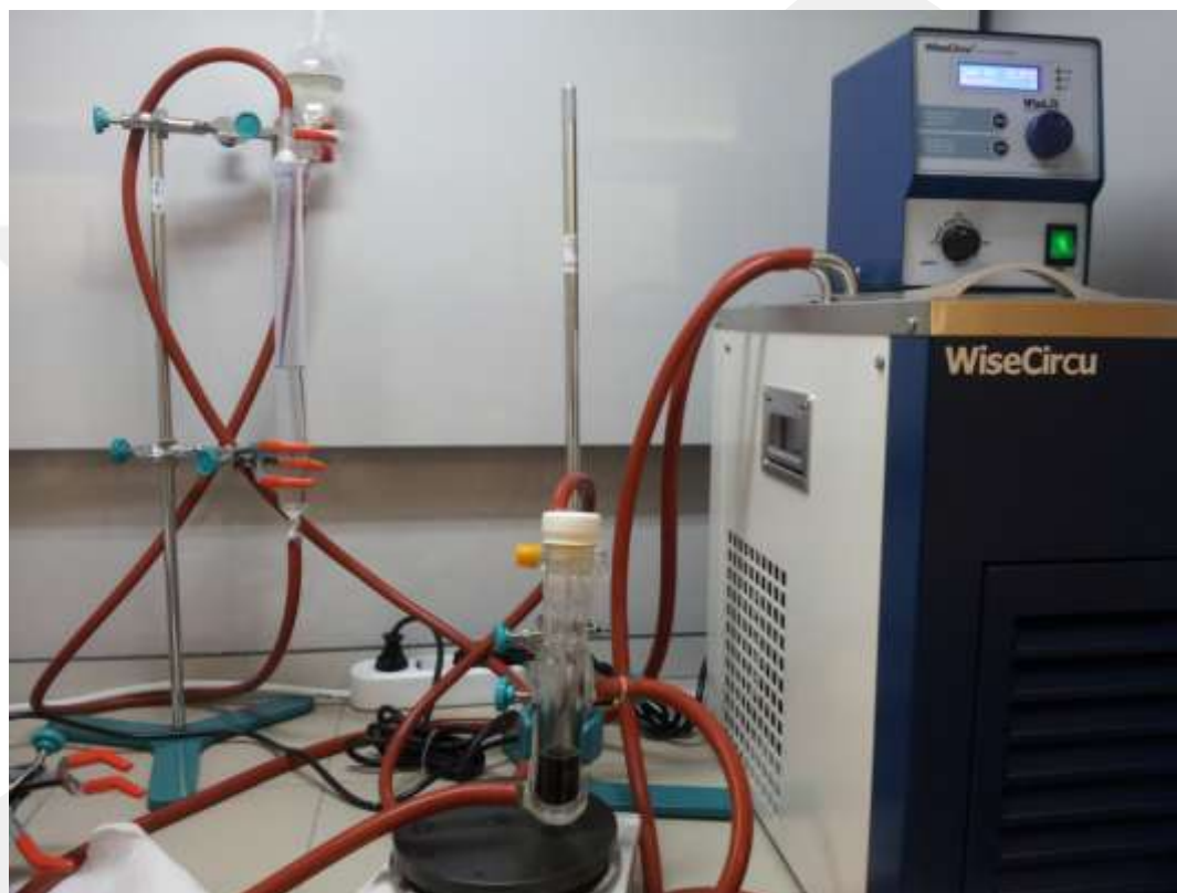
Figure 2.4 System used for the hydrogen generation studies
