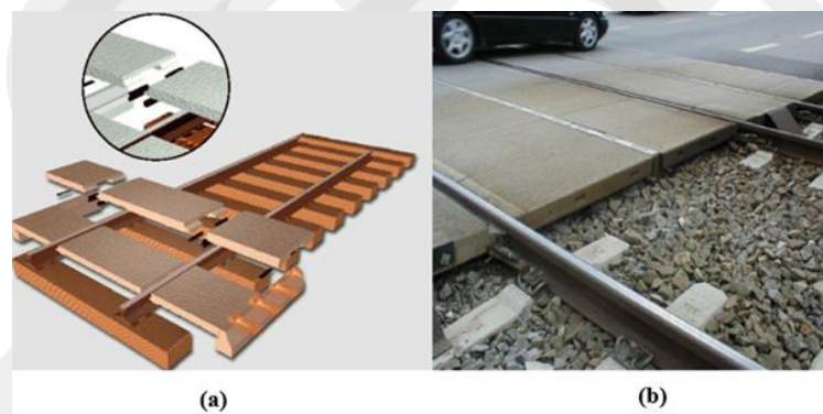
Figure 1.4 (a) Schematic of PC railroad crossing system, (b) Installed PC railroad crossing system [10]
