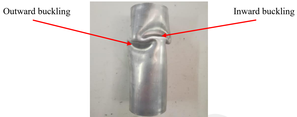
Figure 4.20 Failure mode of HCAT-180-2-1 specimen (D=60 mm)
