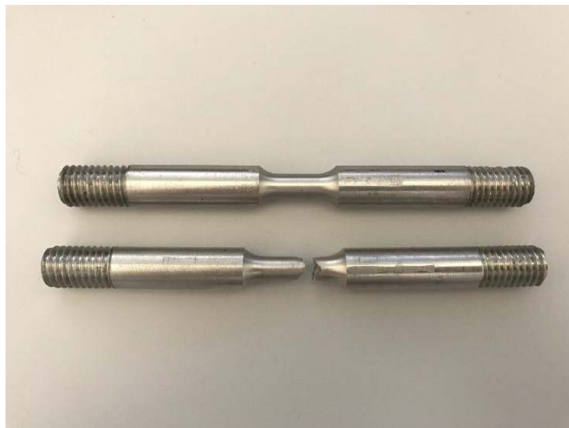
Figure 17. Initial and Ruptured Tensile Test Specimen
