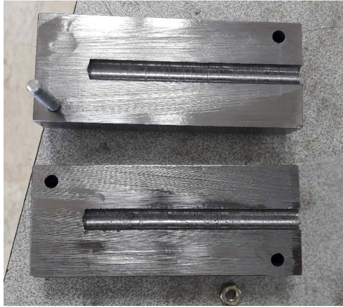
Figure 14. Permanent Steel Mold for Casting Sn-Bi Alloy
