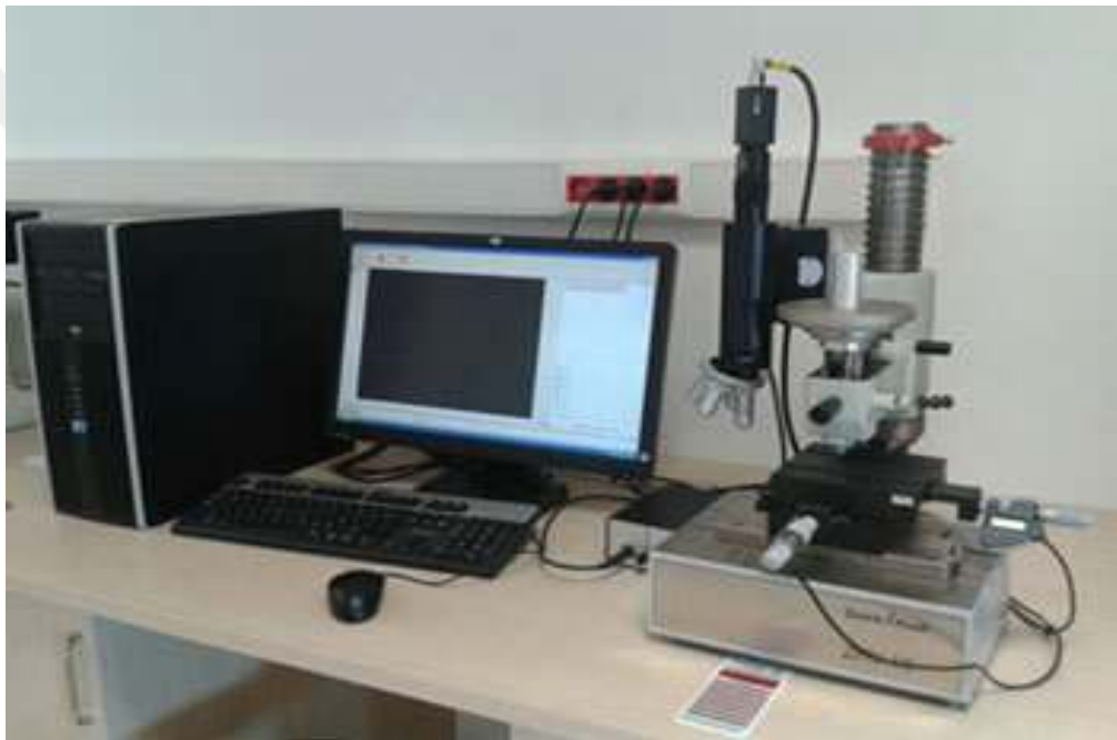
Figure 18. Hardness Measurement Test Device
