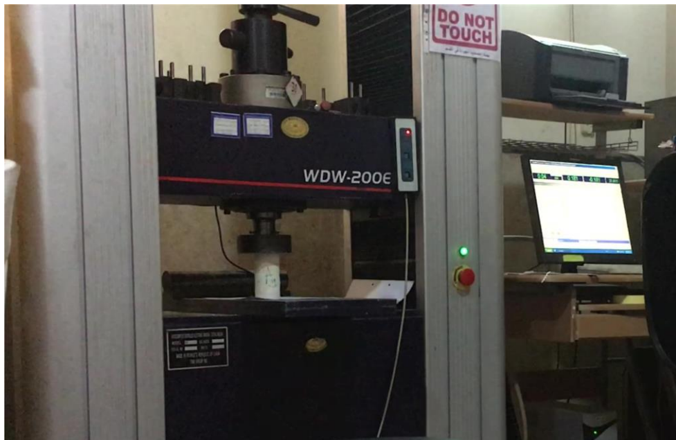
Figure 3.28 Uniaxial Compression Test device (Microcomputer Controlled Electronic Universal testing machine) Model: WDW-200.
