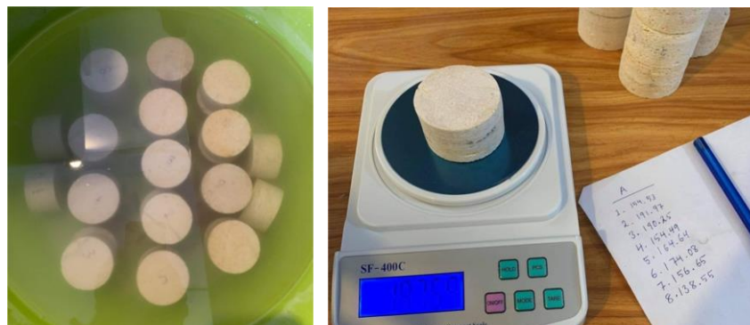
Figure 3.22 Immersion specimens in water for escalating periods of time and weighing each time
