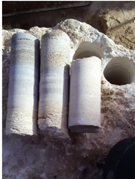
Figure 3.17 Extraction of cylindrical specimens from rock masses
