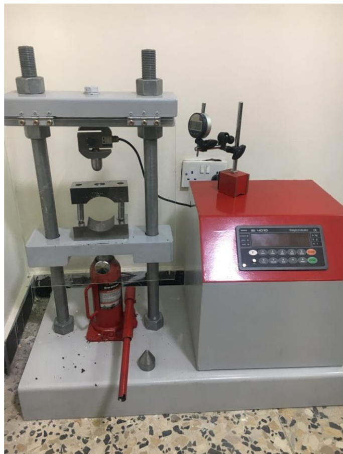
Figure 3.27 Brazilian Test Device
