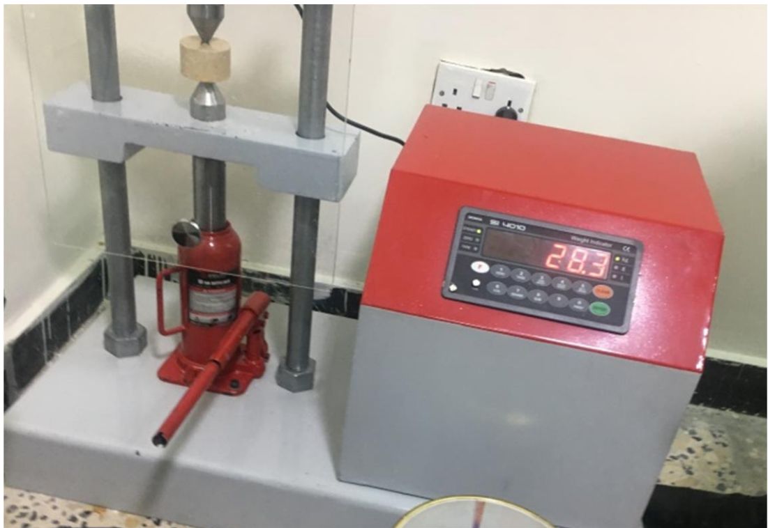
Figure 3.26 Point Load Test Device
