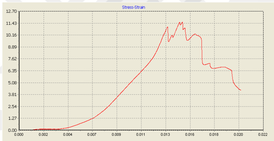
Figure showing the stress-strain relationship of sample B3 in the saturated state
