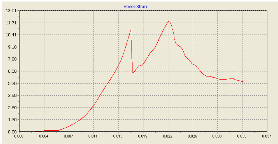
Figure showing the stress-strain relationship of sample B1 in the saturated state
