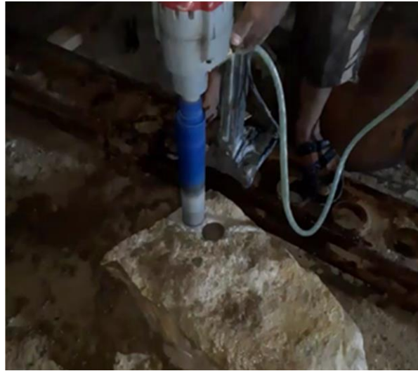
Figure 3.16 Extraction of cylindrical specimens from rock masses
