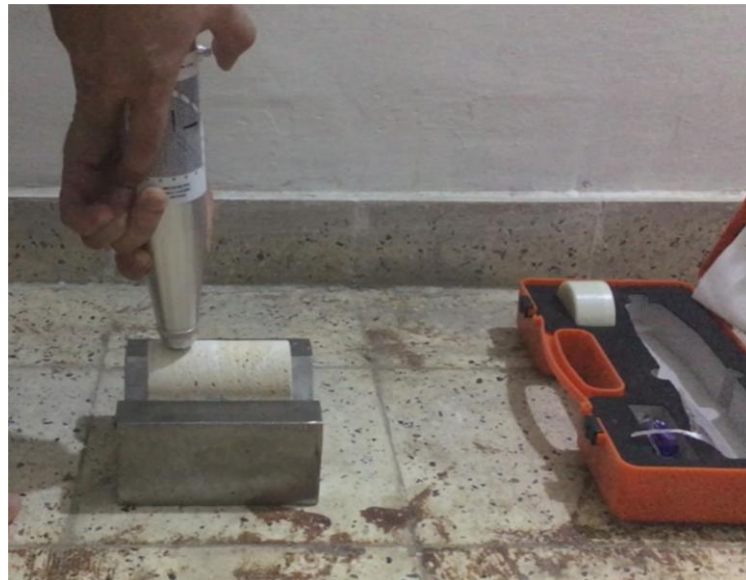
Figure 3.25 Testing the rebound number (Schmidt hammer) of rock specimens
