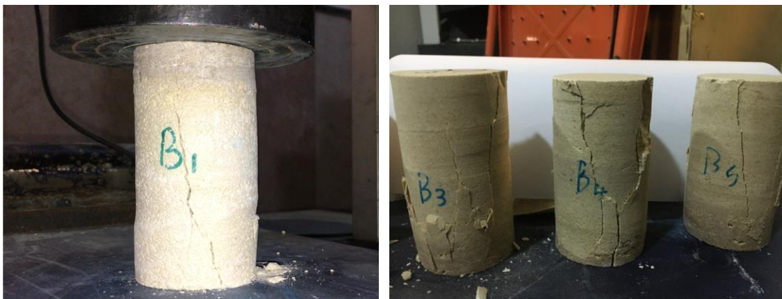
Figure 4.18 Failure modes in dry and saturated conditions of the rock sample B under uniaxial compressive strength
