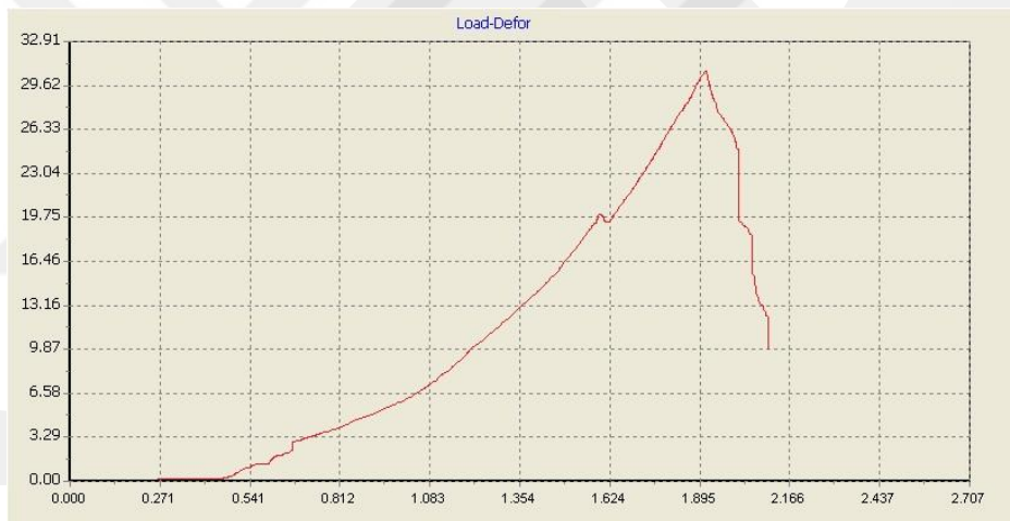
Figure showing the load-deformation relationship of sample A4 in the dry state
