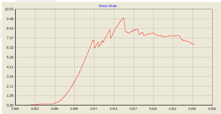
Figure showing the stress-strain relationship of sample C3 in the dry state
