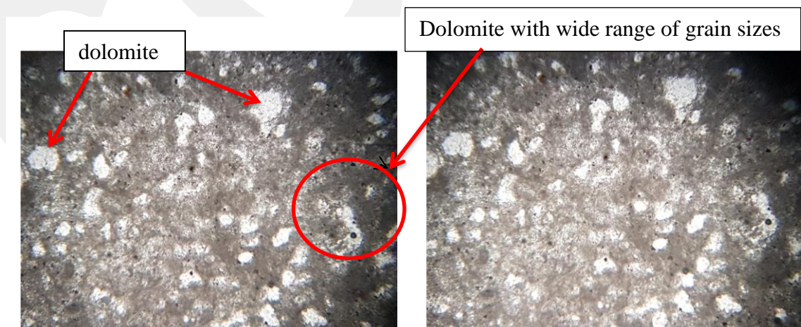
Figure 4.7 Reflect microscope images of rock specimens type ( C )
