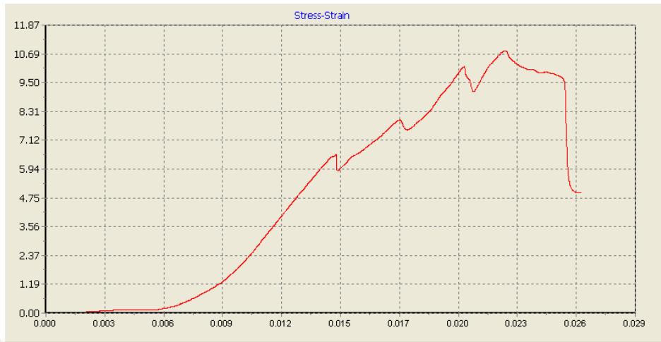
Figure showing the stress-strain relationship of sample C2 in the saturated state
