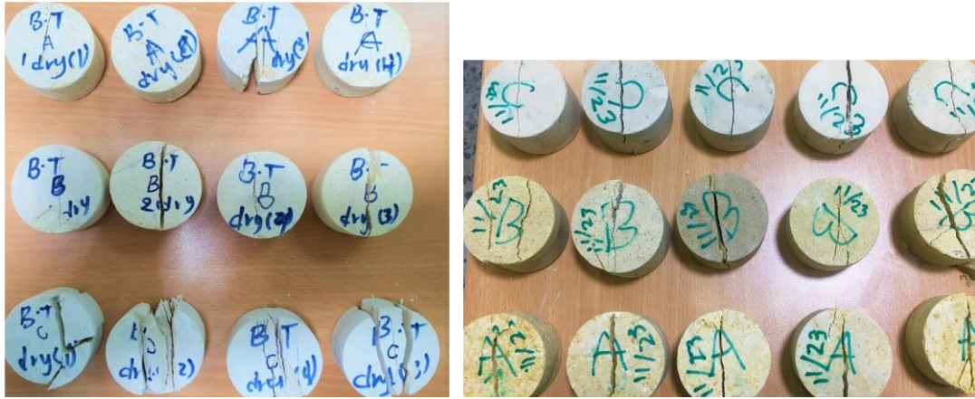
Figure 4.15 Failure modes in dry and saturated conditions of the rock samples A, B, & C under Brazilian test
