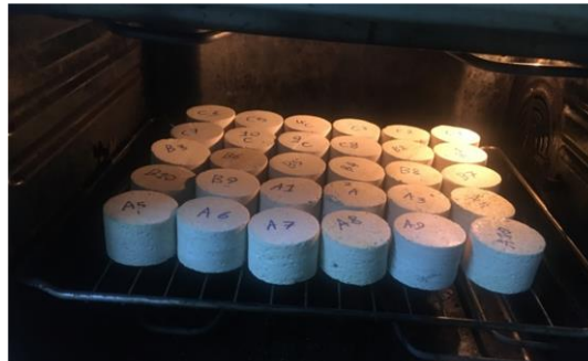
Figure 3.21 Drying and weighing the rock specimens before immersing them in water
