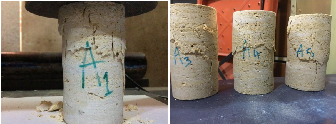
Figure 4.17 Failure modes in dry and saturated conditions of the rock sample A under uniaxial compressive strength
