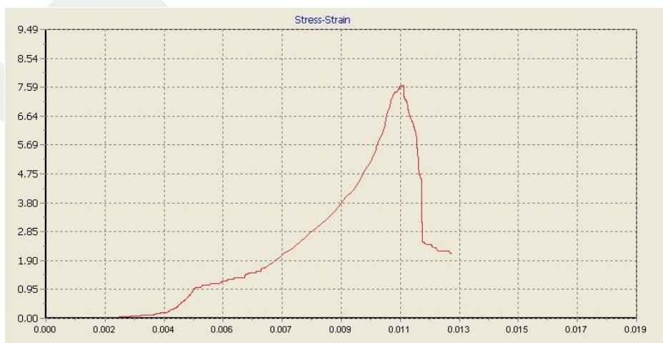
Figure showing the stress-strain relationship of sample A5 in the dry state
