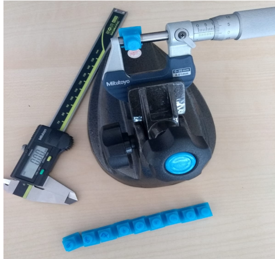
Figure 29 The micrometer instrument
