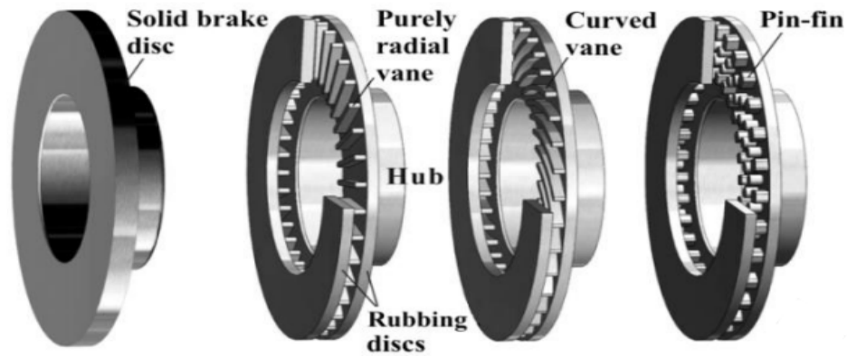
Figure 1.6: Brake disc types. Taken from Mew et. al. [9]
