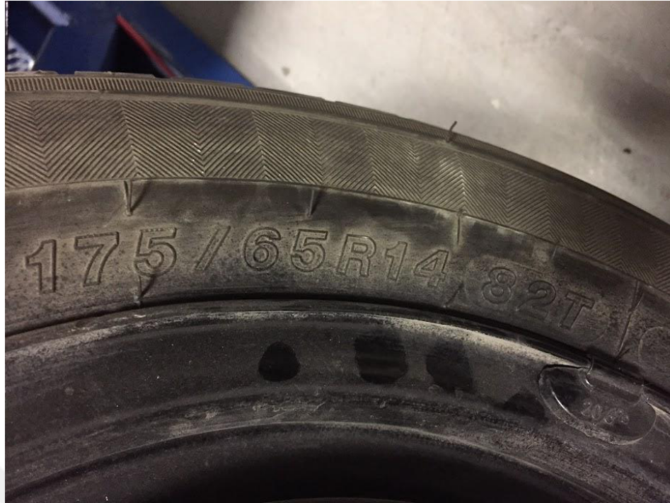
Figure 5.3: Tire codes of the wheel on the experimental setup.
