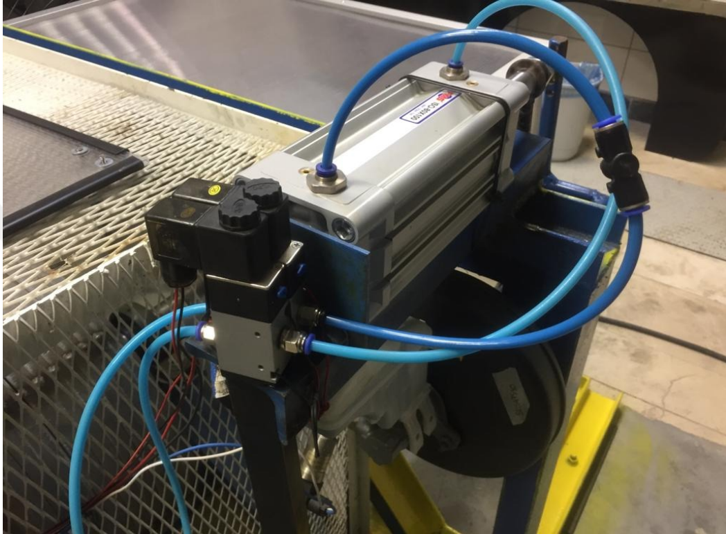
Figure 5.6: Pneumatic piston that creates the braking force and pneumatic valves on the side.
