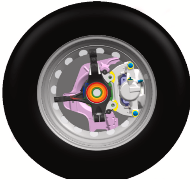
Figure 3.2: Cross sectional view of modeled brake components.
