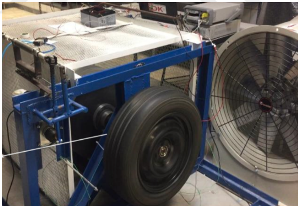
Figure 5.9: Test rig while accelerating the brake components.
