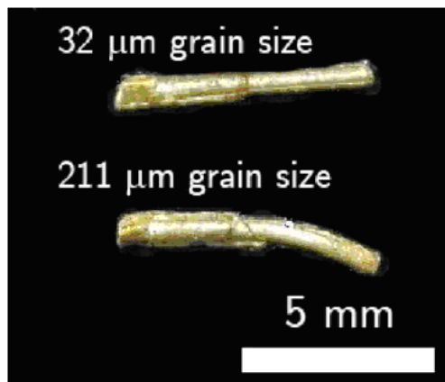
FIGURE 2.2: Curving tendency of extruded micro-pin with different grain size [5]
