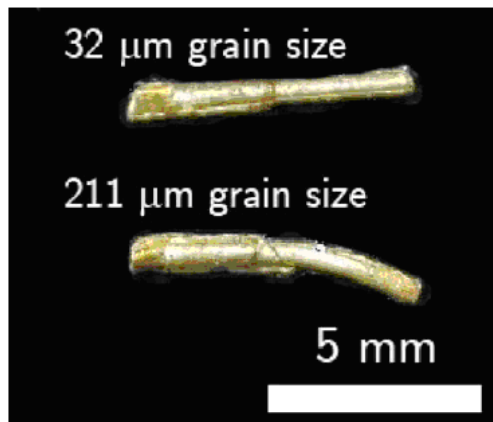
FIGURE 1.5: Curving tendency of extruded micro-pin with different grain size [5]
