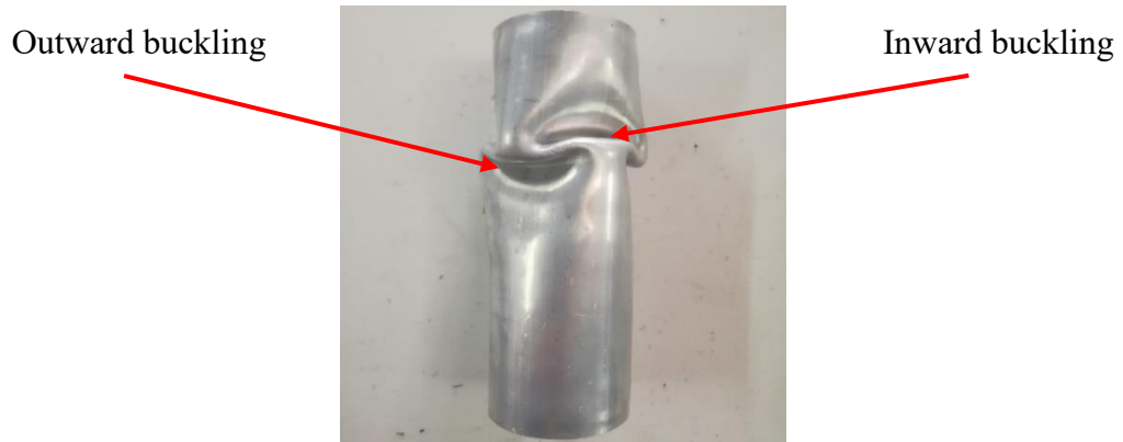
Figure 4.20 Failure mode of HCAT-180-2-1 specimen (D=60 mm)
