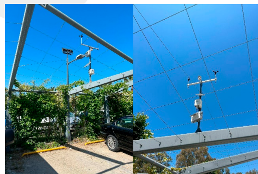
Figure 3. HOBO RX3000 meteorological station installations (Vilayetler Evi on the left, Sasalı Natural Life Park on the right).
